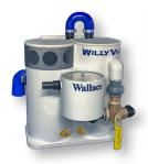
**a.** Willy Vac: Should be installed as low as possible, but no higher than 36 inches from the lowest section of the keel from which you will be vacuuming. You also want to have easy access to the lid/strainer basket, and the diverter valve. The Willy Vac comes with a short power cord connected to a GFI. You will need to connect the boat's power to the 3-pin deutcsh connecter already installed at the end of the GFI box. Mount this level with or below the Willy Vac.
